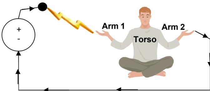
Fig. 1. Conceptual drawing of a corona discharge propagating through the human body, finger tip to finger tip, before returning to its source.
