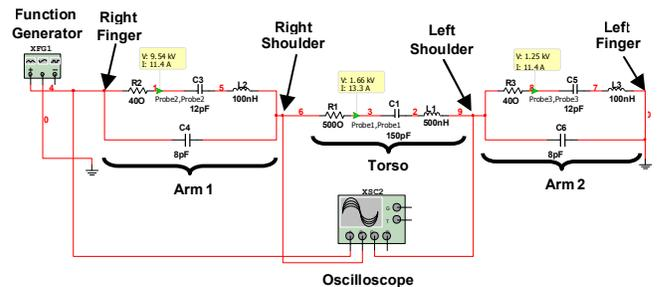
Fig. 2. Electrical schematic for modelling the situation shown in Fig.1.
