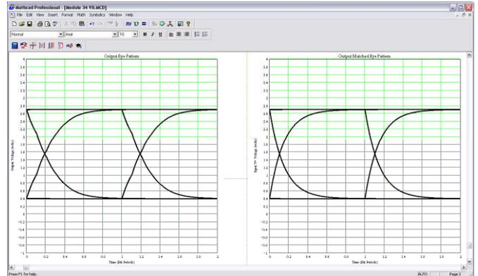
Fig. 4. 55Mbps load eye pattern for the actual CMOS driver (left), and the hypothetical driver (right). The transmission line impedance is  $113\Omega$ , which is close to  $R_{LOW}$ .  $R_{HIGH}$  is still equal to  $287.5\Omega$ .
