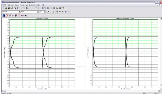
Fig. 1. 55Mbps load eye pattern for the asymmetrical CMOS driver (left), and the hypothetical symmetrical driver (right). The transmission line impedance is  $194\Omega$ , which is the average of  $R_{HIGH}$  and  $R_{LOW}$ .
