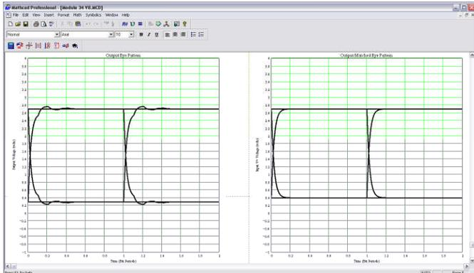
Fig. 2. 55Mbps load eye pattern for the asymmetrical CMOS driver (left), and the hypothetical symmetrical driver (right). The transmission line impedance is  $287.5\Omega$ , which is equal to  $R_{HIGH}$ .
