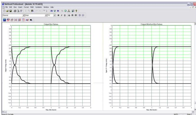
Fig. 3. 55Mbps load eye pattern for the asymmetrical CMOS driver (left), and the hypothetical symmetrical driver (right). The transmission line impedance is  $113\Omega$ , which is close to  $R_{LOW}$ .
