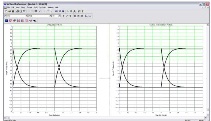
Fig. 5. 55Mbps load eye pattern for the actual CMOS driver (left), and the hypothetical driver (right). The transmission line impedance is  $113\Omega$ , which is close to  $R_{LOW}$ , and  $R_{HIGH}$  has been lowered to  $175\Omega$ , while the driver risetime has been reduced from 5.5ns to 3.5ns.
