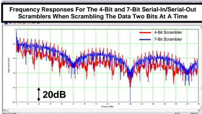
Fig. 14. Frequency responses when scrambling the input data two bits at a time.
