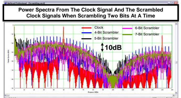
Fig. 6. Power spectra from scrambling a 50MHz clock signal two bits at a time with 4-bit, 5-bit, 6-bit, and 7-bit scramblers.
