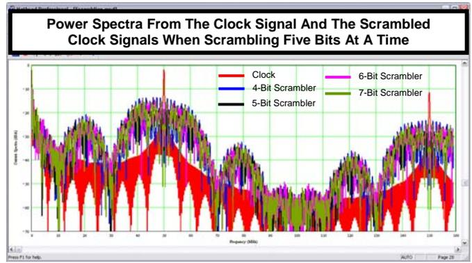
Fig. 12. Power spectra from scrambling a 50MHz clock signal five bits at a time with 4-bit, 5-bit, 6-bit, and 7-bit scramblers.
