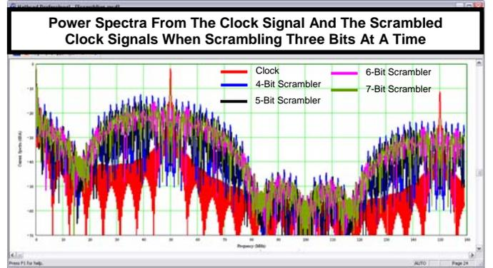
Fig. 8. Power spectra from scrambling a 50MHz clock signal three bits at a time with 4-bit, 5-bit, 6-bit, and 7-bit scramblers.
