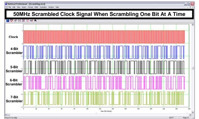
Fig. 3. Scrambling a 50MHz clock signal one bit at a time with 4-bit, 5-bit, 6-bit, and 7-bit scramblers, and when  $f_{\max} = 100\text{MHz}$ .
