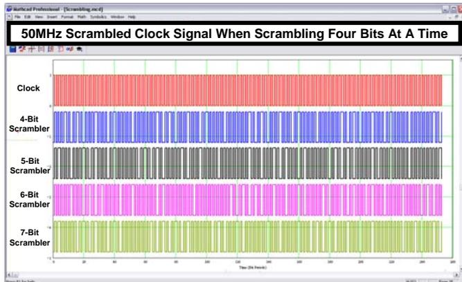
Fig. 9. Scrambling a 50MHz clock signal four bits at a time with 4-bit, 5-bit, 6-bit, and 7-bit scramblers, and when  $f_{max} = 100\text{MHz}$ .
