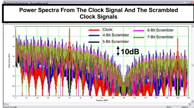
Fig. 4. Power spectra from scrambling a 50MHz clock signal one bit at a time with 4-bit, 5-bit, 6-bit, and 7-bit scramblers.
