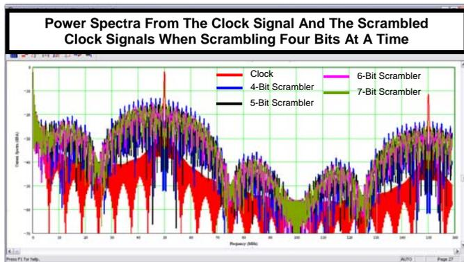
Fig. 10. Power spectra from scrambling a 50MHz clock signal four bits at a time with 4-bit, 5-bit, 6-bit, and 7-bit scramblers.
