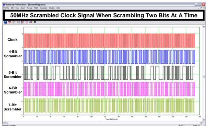
Fig. 5. Scrambling a 50MHz clock signal two bits at a time with 4-bit, 5-bit, 6-bit, and 7-bit scramblers, and when  $f_{max} = 100\text{MHz}$ .
