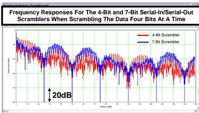
Fig. 16. Frequency responses when scrambling the input data four bits at a time.
