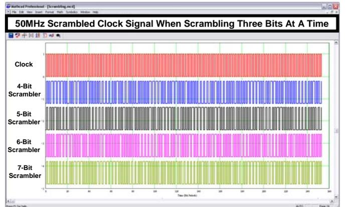
Fig. 7. Scrambling a 50MHz clock signal three bits at a time with 4-bit, 5-bit, 6-bit, and 7-bit scramblers, and when  $f_{max} = 100\text{MHz}$ .
