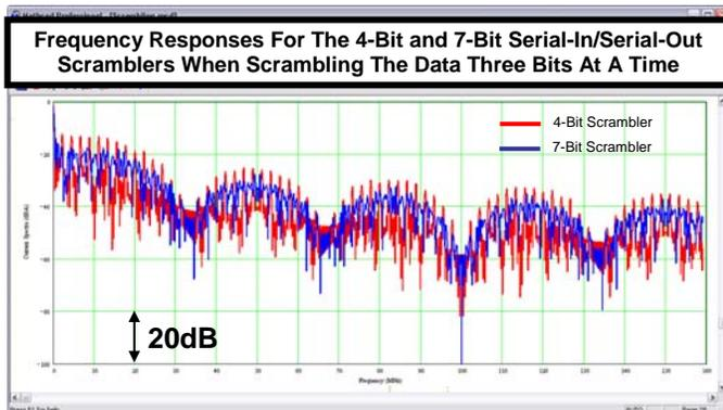
Fig. 15. Frequency responses when scrambling the input data three bits at a time.
