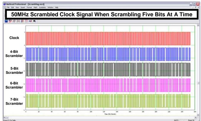
Fig. 11. Scrambling a 50MHz clock signal five bits at a time with 4-bit, 5-bit, 6-bit, and 7-bit scramblers, and when  $f_{max} = 100\text{MHz}$ .
