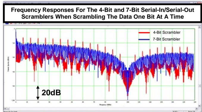
Fig. 13. Frequency responses when scrambling the input data one bit at a time.
