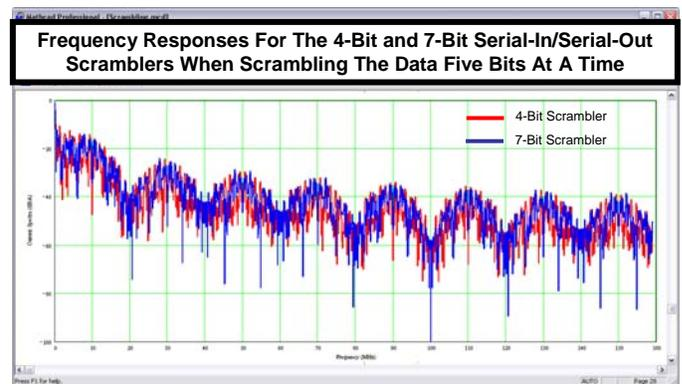
Fig. 17. Frequency responses when scrambling the input data five bits at a time.
